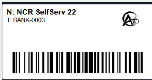
Printed to a Zebra over ZPL — asset name, tag and barcode
